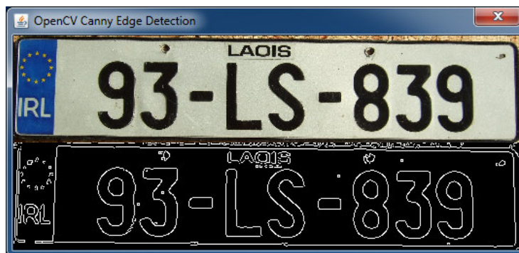
Figure 22 Canny edge detection with lower bounds = 127, upper bounds = 255, aperture size = 3, and L2 gradient = false
