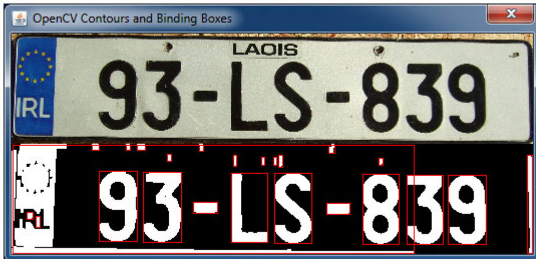
Figure 35 Refined binding boxes of a licence plate
