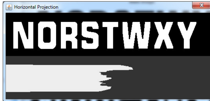
Figure 23 Example of a horizontal projection
