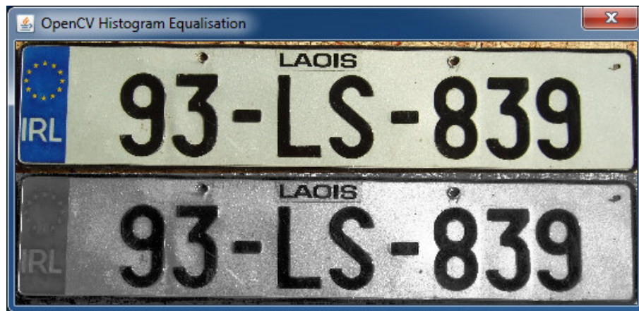
Figure 13 Original image and greyscale version after equalisation
