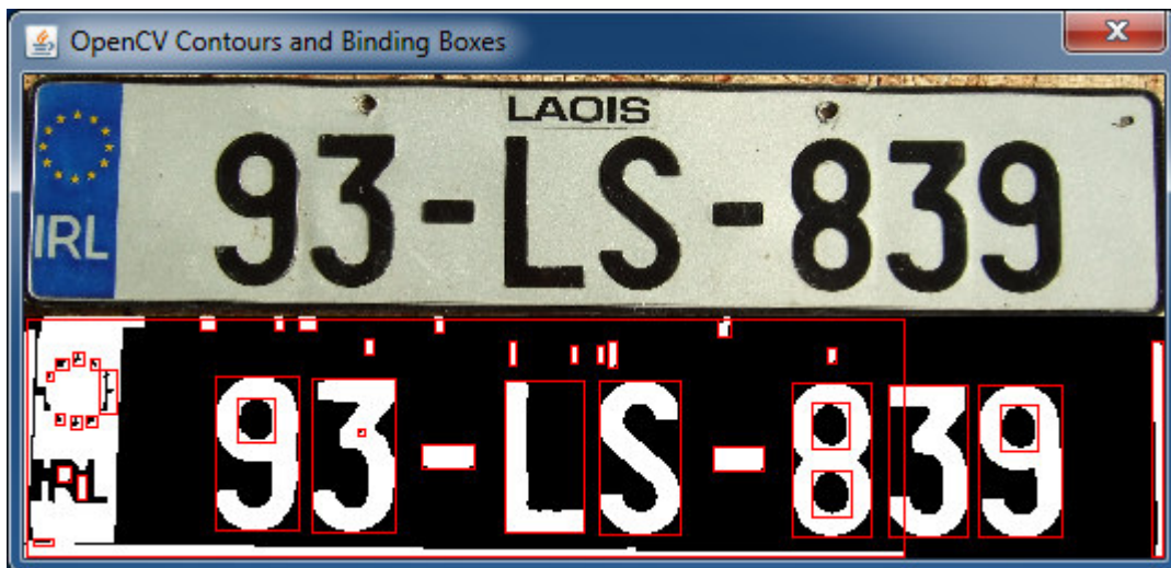
Figure 34 Binding boxes of a licence plate
