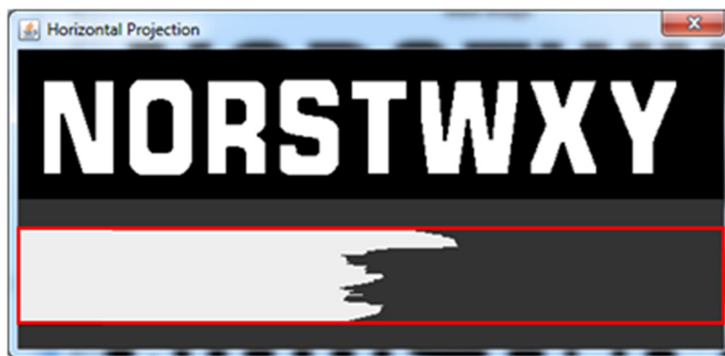
Figure 25 The area of interest in the horizontal projection
