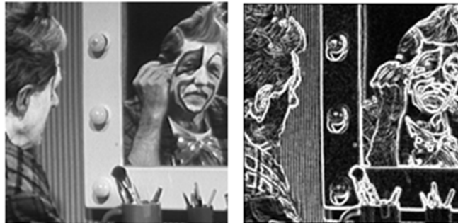
Figure 19 Original image (left) and Sobel applied (right)
