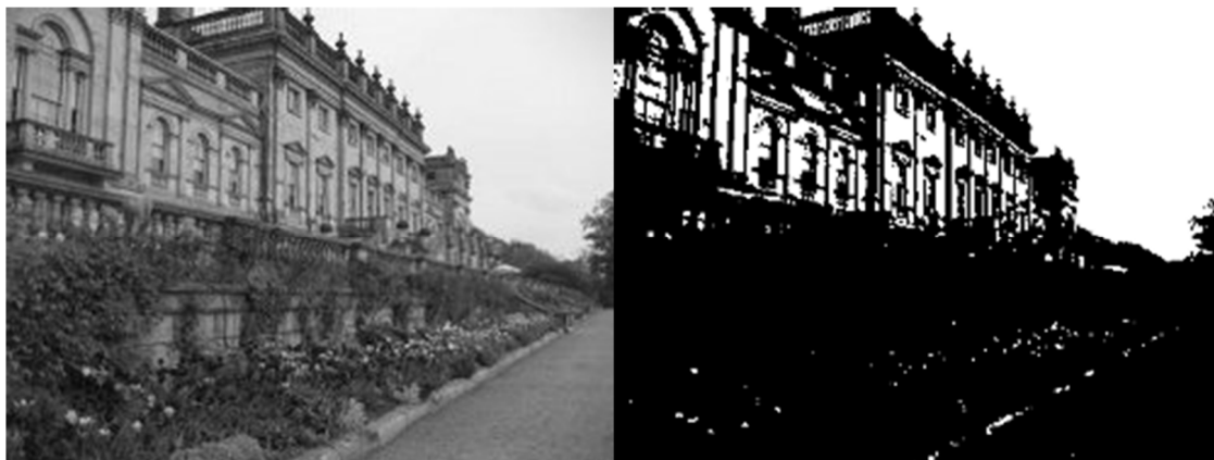
Figure 16 Image before and after Otsu thresholding
