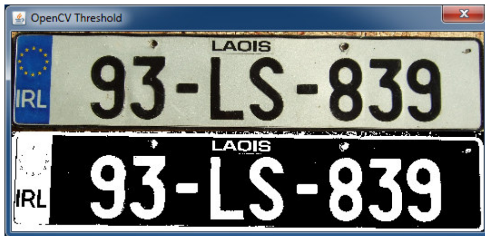
Figure 14 Thresholding using grey image, lower bound of 127, and upper bound of 255
