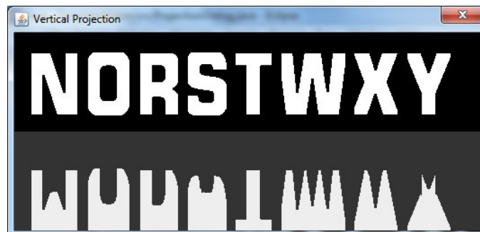
Figure 24 Example of a vertical projection
