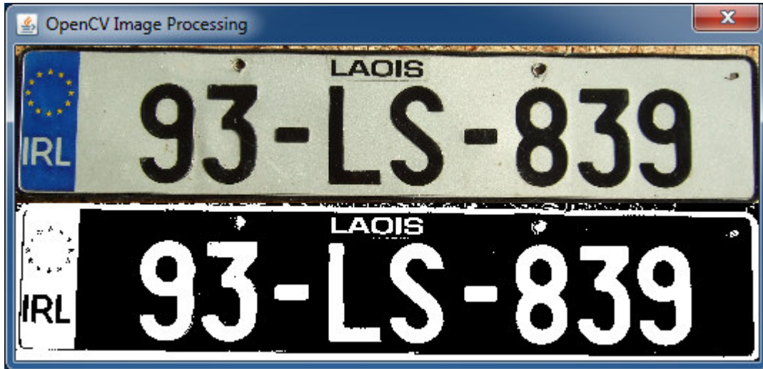
Figure 17 Image before and after Otsu thresholding with a value of 118
