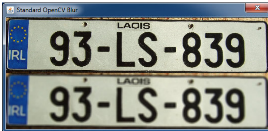
Figure 5 8 Standard OpenCV blur with kernel size = Size (5, 5)
